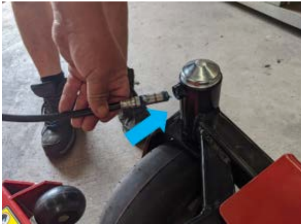
Front wheel grease nipples (2)
