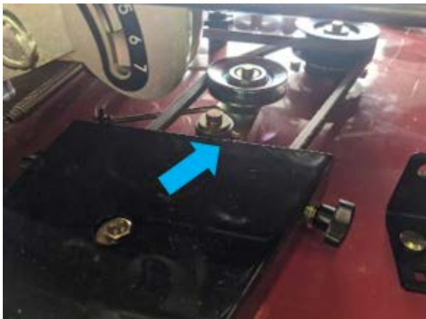
Hydro Gear weldment grease nipple (1)
